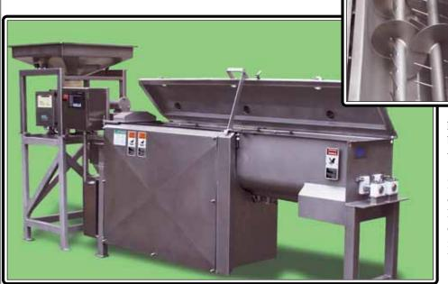
Blentech has developed the first truly continuous, full absorption rice cooker for Asian 'sticky' rice, flavored rice pilaf or any grain product where controlling the percentage of water content in the hydrated product is critical to quality. The HydraTherm system with process and machine patents pending, continuously feeds raw rice into the inlet and perfectly hydrated, completely cooked steamed rice continuously feeds out the discharge opening.
