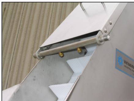
Spray bar gives product final rinse and provides tank makeup water.
