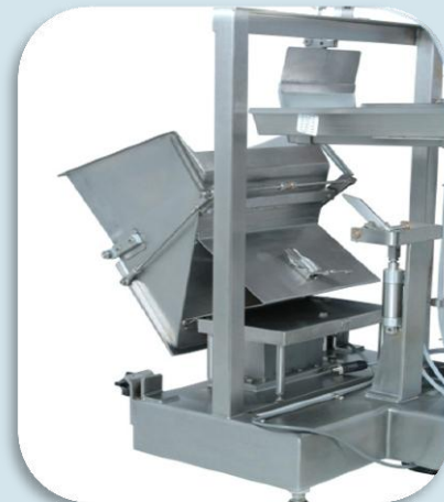
Tool-less removal of contact parts
