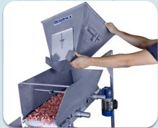
Tool-less removable hopper
